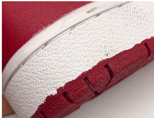
Color bleeding over the outsole parting line. The shoe is also dirty. There is a little over gluing on the outsole.
