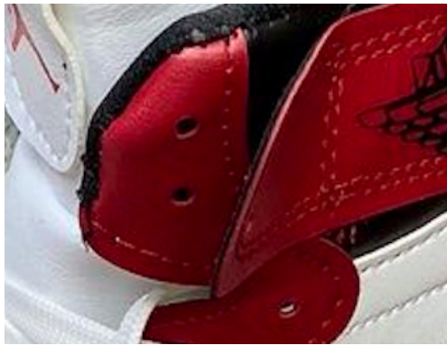
Poorly turned seam is lumpy and mis-shapen.
