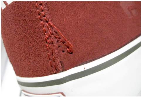
Rubber blooming - chemicals inside the rubber are leaching out.
