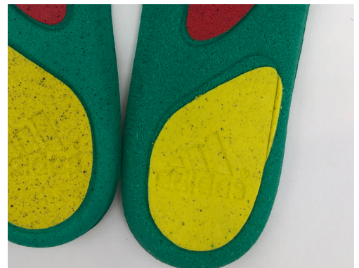
Color bleeding. The foam insert is not fitting in it's space.
