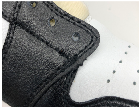
Rough stitching caused by poor workmanship.
