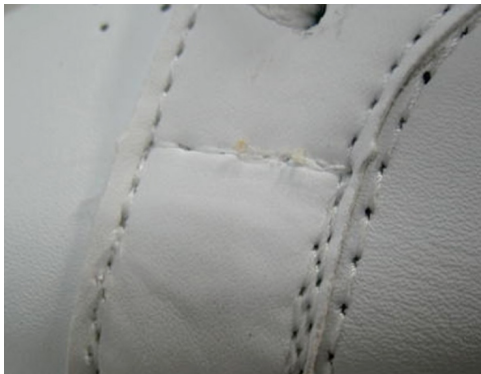
Melted thread balls.
