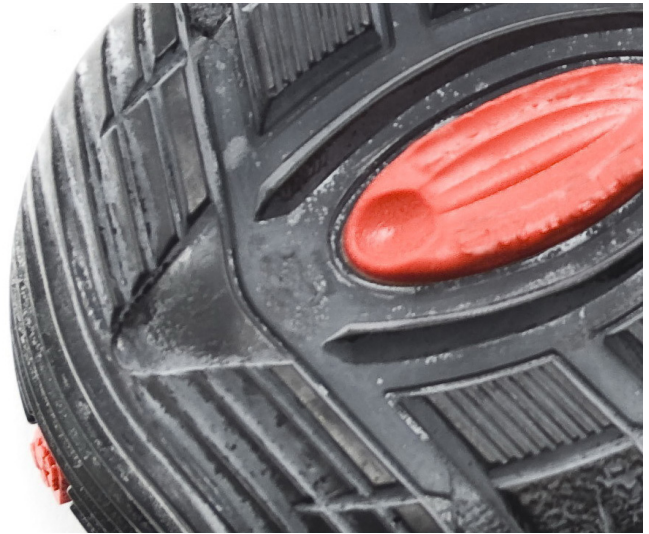
Rubber blooming - chemicals inside the rubber are leaching out.
