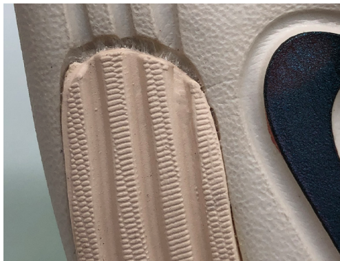
Parts don't fit together, cheap molds and poor stock fitting.
