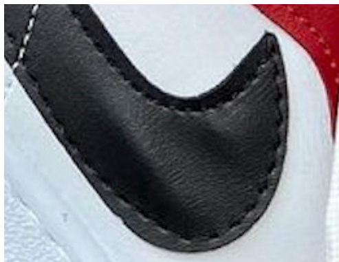
Rough stitching, not following the edge
