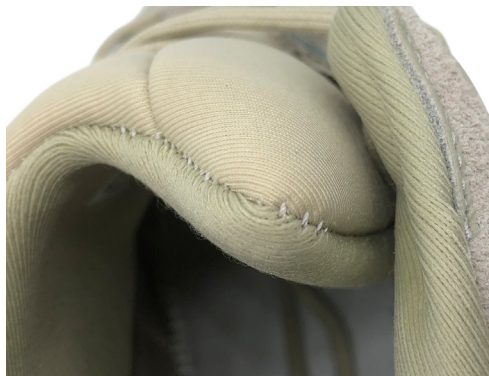
Turned out seams with stitching showing
