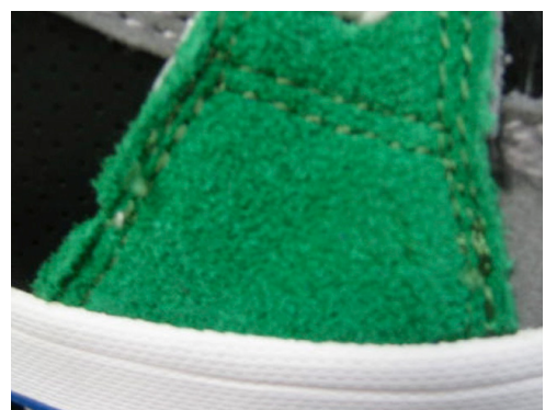
Rough cutting caused by dull cutting dies.
