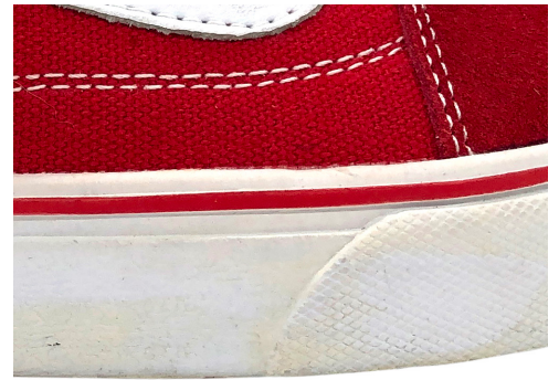
Painted rubber. Unstable rubber is yellowing in UV light.
