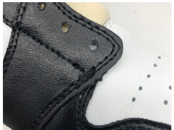
Rough stitching caused by poor workmanship.
