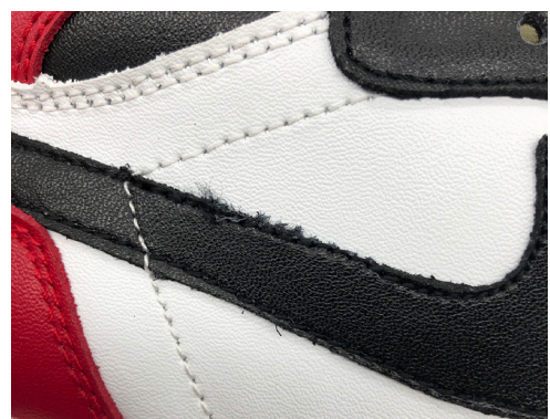
Rough cutting caused by dull cutting dies.
