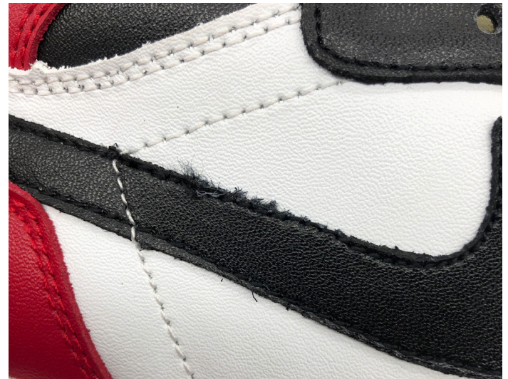
Rough cutting caused by dull cutting dies.
