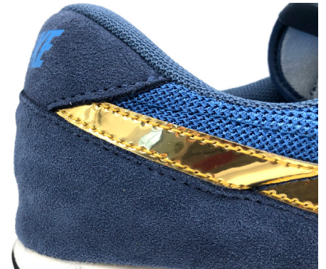
Wrinkles and mis-shaped heel counter are proof of being improperly molded.
