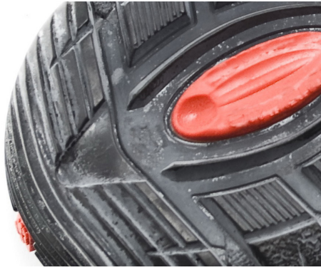
Rubber blooming - chemicals inside the rubber are leaching out.
