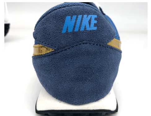
Upper is twisted or "clocked" during lasting operation.
