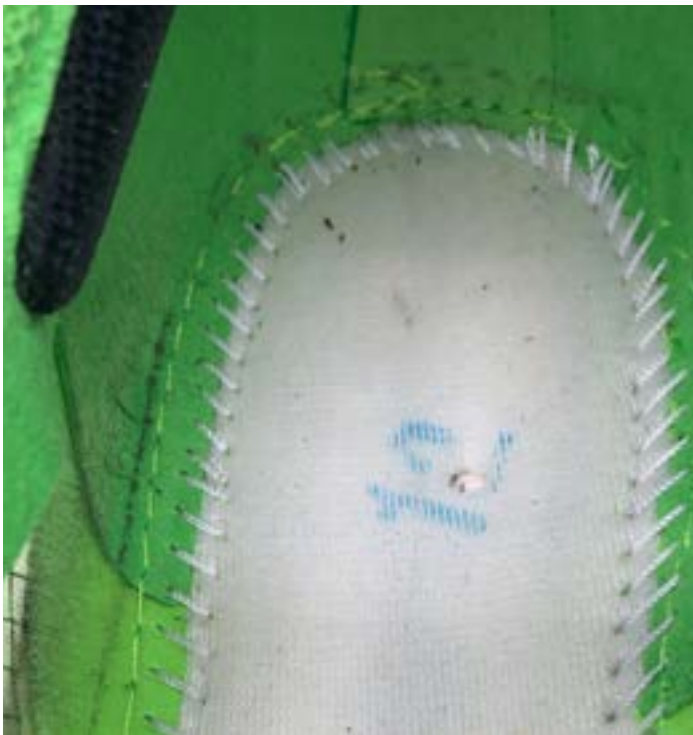
This is what the Strobel sock looks like inside the shoe. You will need to lift the footbed to see the stitching.
