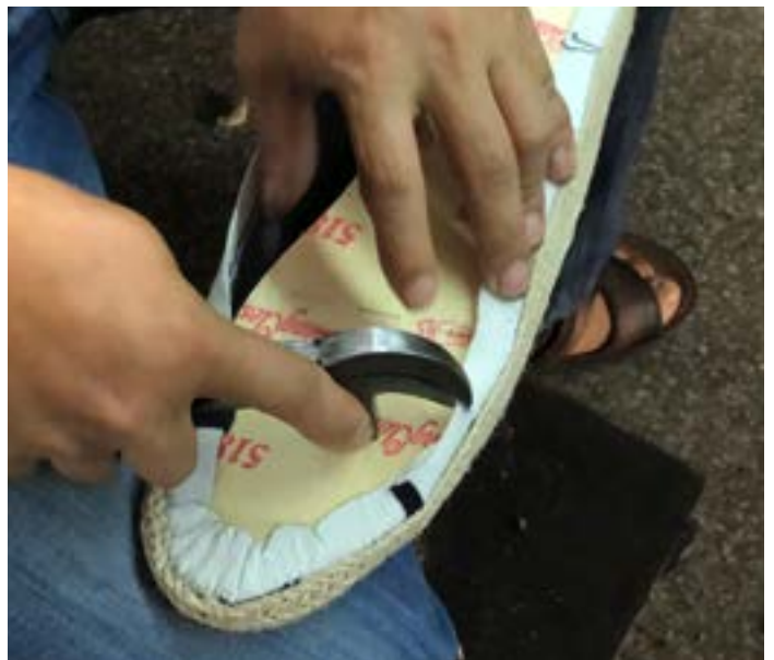
Here a worker is using lasting pliers to wrap the upper over the edge of a lasting board.
