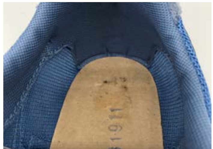
This is what a board lasted shoe looks like inside - no edge stitching.
