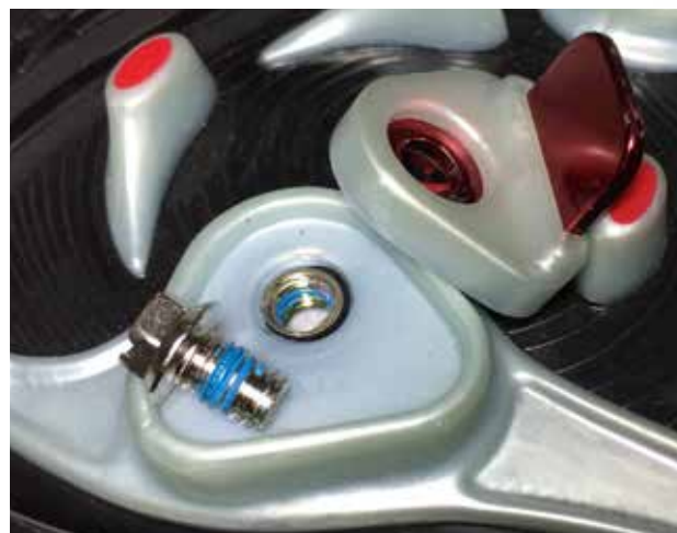
Insert molded 316 stainless steel threaded insert. M5 screw with Loctite™ thread compound to prevent loosening.
